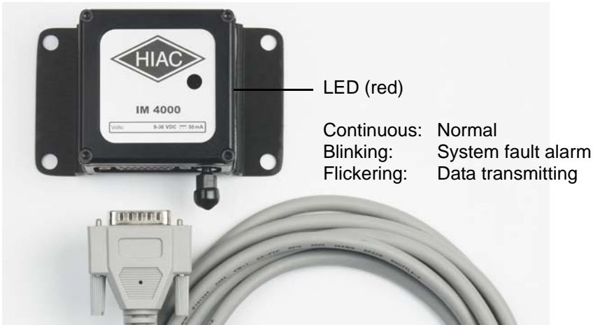
Fig 5-7: IM4000-3 Indicator Location
