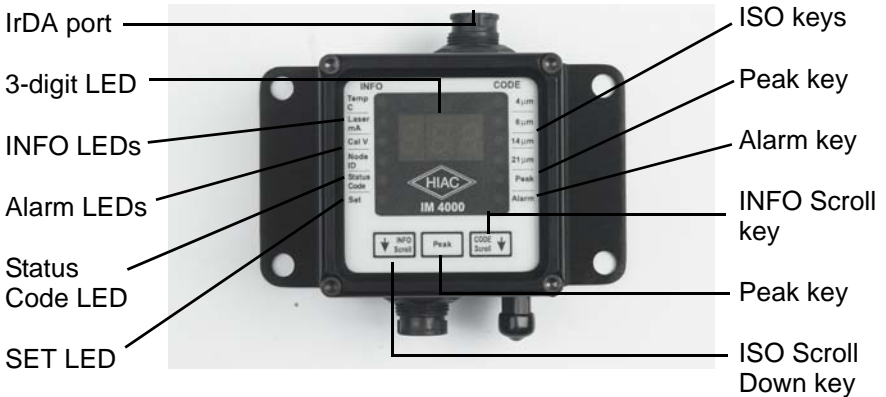
Fig 5-8: IM4000-4, -5 and PT4000-0, -4, -5, -6, -8 Indicators and Controls (IM4000 shown)
